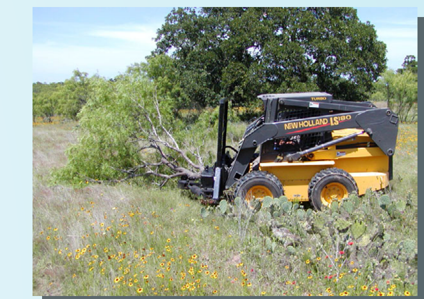
Hydraulic tree shearing has become a popular brush control method. Soil disturbance is minimized.
