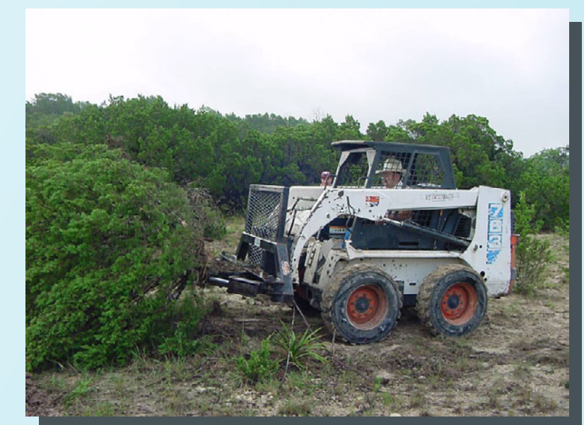
Hydraulic tree shearing has become a popular method for selective brush removal.
