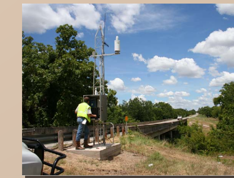
Photo 9. An LCRA Hydromet streamflow gauge is situated on Wilbarger Creek at FM 1704 downstream of Elgin.
