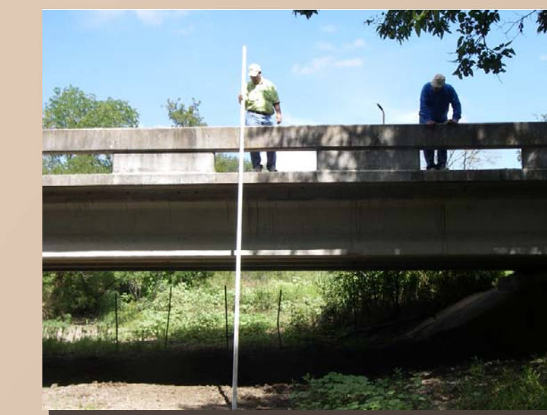
Photo 8. LCRA staff measures stream channel cross-sections at Lower Dry Creek at Upper Elgin Road. This view looks upstream.
